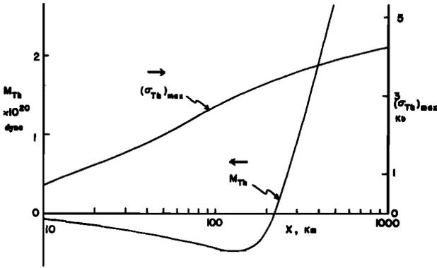
Fig. 3. Thermal bending moment and maximum thermal stress in the cooling lithosphere as a function of the distance from the ridge crest.
