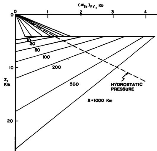
Fig. 2. Thermal stresses in the cooling lithosphere as a function of depth at several distances from the ridge crest.
