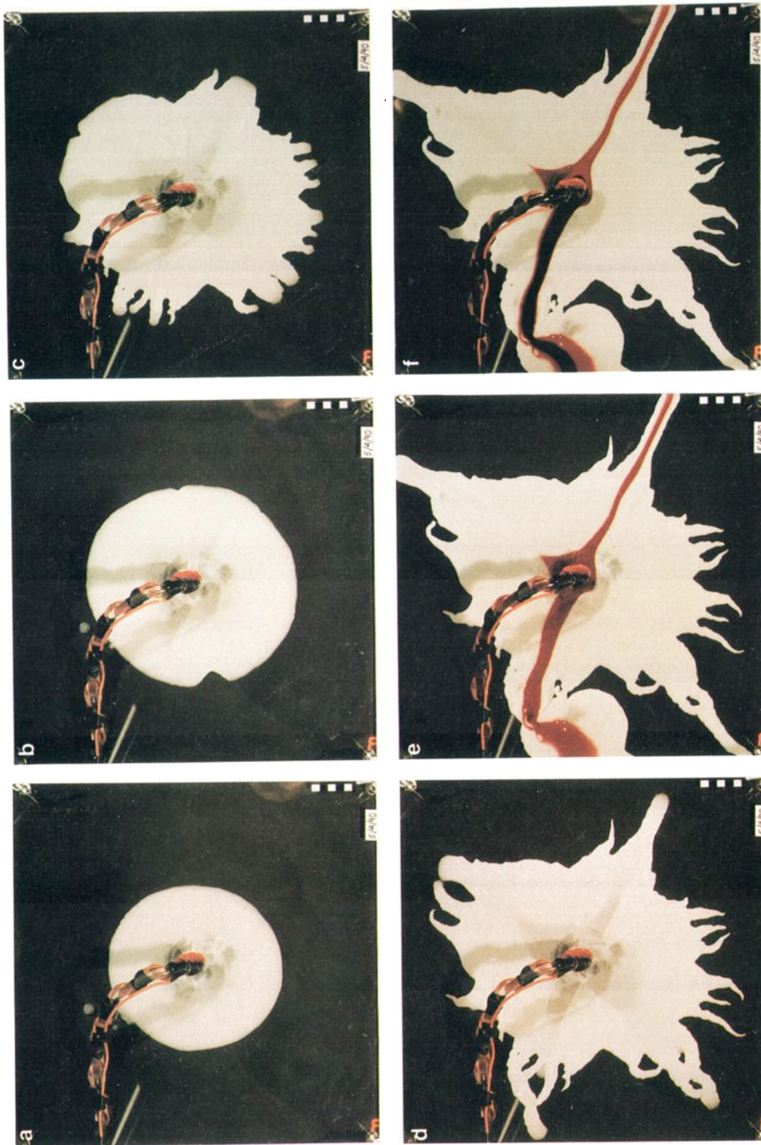
Plate 1. Photographs of the evolution of paraffin flowing with constant volume flux through a cooled slot from a point source. From left to right: (a) At 12 s after start of the experiment a circular intrusion is seen. (b) At 16 s two small notches have grown. (c) By 20 s numerous fingers break out. (d) At 24 s the fingers have grown considerably. (e) At 52 s, dye reveals there is flow through two channels; there is also evidence that third channel stopped just as the dye entered the tank. (f) At 92 s, darker dye reveals that there is flow in only one channel.
