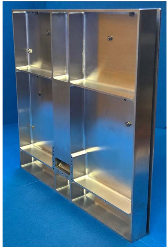
Figure 18. An 8 \times 8 element subarray of the high-gain antenna with the ultrasonic additively manufactured backplate.
