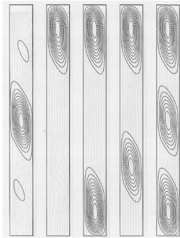
Figure 12: Different stable time-independent spatially localized structures in doubly diffusive convection in a rectangular cavity obtained for identical parameter values. The solutions are visualized using streamlines of the flow. From [14].
