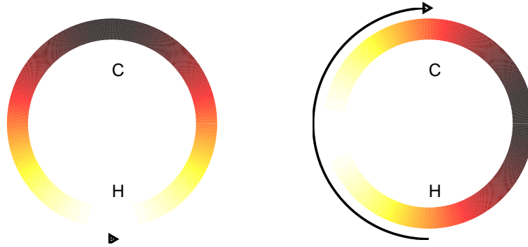
Figure 10: Fixed point solutions for convection with \chi = 90 with (a) r = 0.1 and (b) r = 100 . “H” and “C” indicate locations of heating and cooling along the loop. The colors indicate the temperature pattern for a fixed point in the system. Arrows indicate direction and relative magnitude of circulation.
