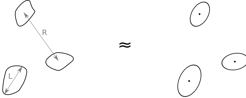
Figure 3: Approximation of vortex patches as ellipses under the moment model of MZS.
