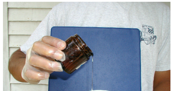
Experiments from the porch: an open siphon with Anshuman's Boger fluid
