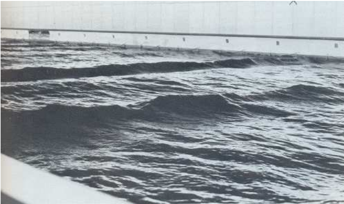
Figure 1: Wavetrain in deep water ( L = 2.3 m, h = 7.6 m), with 60 meters between photos.
