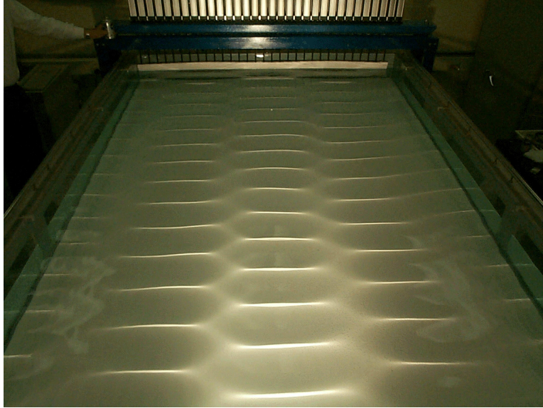
Figure 4: Experimentally stable wave patterns in deep water. Frequency=3Hz, wavelength=17.3cm.
