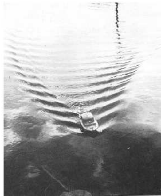
Fig. 5.9 – Ship waves on deep water. Photographing a model gives a more dramatic pattern than a full size ship. If the boat is not obviously a model the capillary waves in front show the scale clearly.
