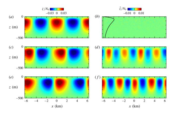
Snapshots from simulation at Nt=0 (top), 200 (middle) and 400 (bottom) with the total horizontal velocity field (left) and the horizontal velocity having subtracted that of the primary wave (right)
