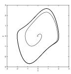
Figure 2: Sample state-space orbit of the Van der Pol oscillator for  $\mu = 1$ , starting near the unstable origin and converging to the periodic orbit.
