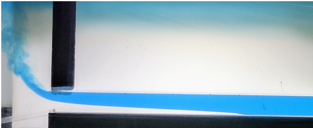
Figure 4: A closeup image of a part of the rectangular channel during an experiment. Here, a salt wedge is observed in the lower half of the tube. For reference, the height of the tube is 2.1 cm
