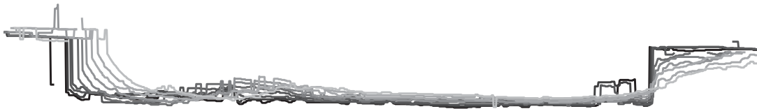
Figure 6: Measured side profiles of 32.5 cm long ice block immersed in fluid moving at U = 3.5 cm s ^{-1} . The edge detection works poorly as a result of the similar colour of the ice block and the dyed melt water. Contours are taken at one minute intervals.
