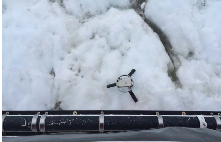
Figure 3: Picture of a GPS tracker placed on the surface of a large iceberg in the Sermilik Fjord (South-East Greenland) from a helicopter. (Photo by F. Straneo)
