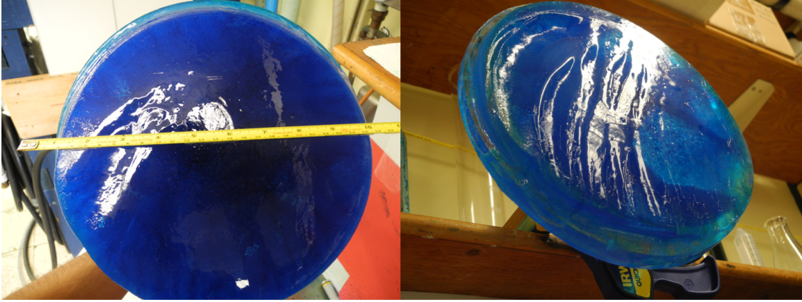
Figure 11: Two pictures of the bottom of the ice blocks after two experiments with the same free stream velocity U = 4 \text{ cm s}^{-1} . In the left panel the rotation rate was lower than the one in the right panel and, in particular, a partial TC was observed in the experiment of the right picture, which was not the case in the experiment of the left one. Wider and deeper elongated melted stripes are visible in the right panel, due to the increased velocity at the base of the ice block determined by the TC dynamics.
