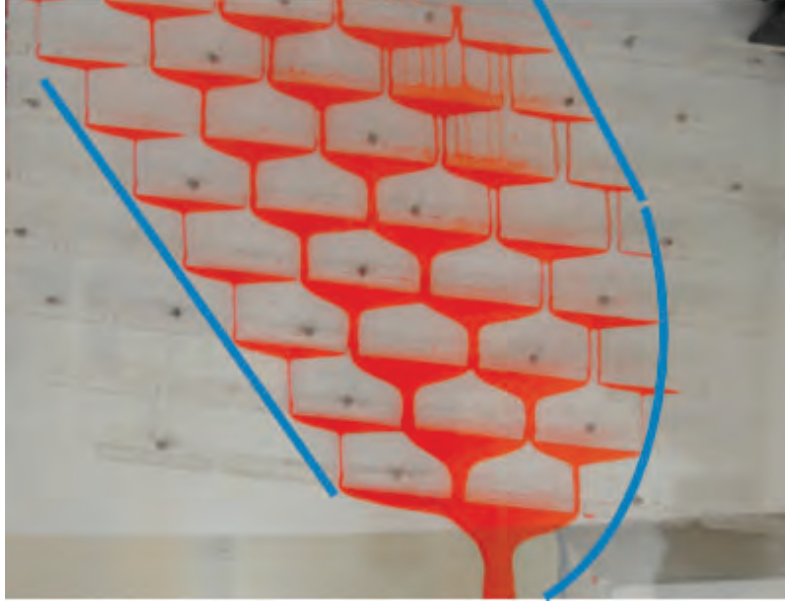
Figure 18: Plumes propagating through an angled array of barriers exhibit a preferred horizontal direction.
