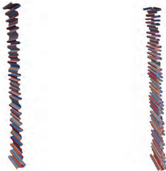
Figure 3.3: Evolution of the perturbation to the interface for two OpenFoam runs with \epsilon = 2.5 \times 10^{-5} \times \frac{a}{r_0} , \mathcal{A} \simeq -0.018 and \text{Ek} \sim 1.6 \times 10^{-5} at \Omega = 2\pi rad/s (left) and 4\pi rad/s (right) demonstrating the effect of increasing rotation on the emergence of smaller scales in the growth of the perturbations.
