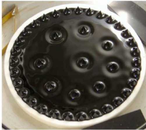
Figure 5: Two-dimensional localized structures on the surface of a ferrofluid. From [23].
