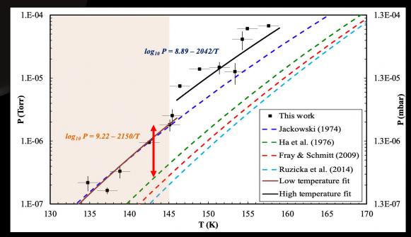
Experimental vapor pressure measurements of benzene ice (black) compared with extrapolations from higher temperature data in the literature (Dubois et al. 2021). Note the large difference (red arrow) between current measurements and the red dashed line, which is the most-commonly used parameterization.
