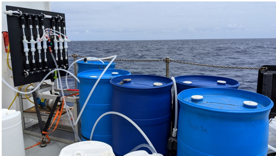
Figure 5.1: Custom large volume POM concentrator used on PARAGON I to collected SPM samples. The seven hollow fiber filters (white) retain particles larger than 0.1 \mu\text{m} .
