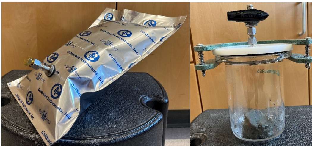
Figure 5.S1: Degassers tested to extract gas from marine sediments: a Calibrated Instruments Cali-Bond bag, and b glass degasser with O-ring seal
