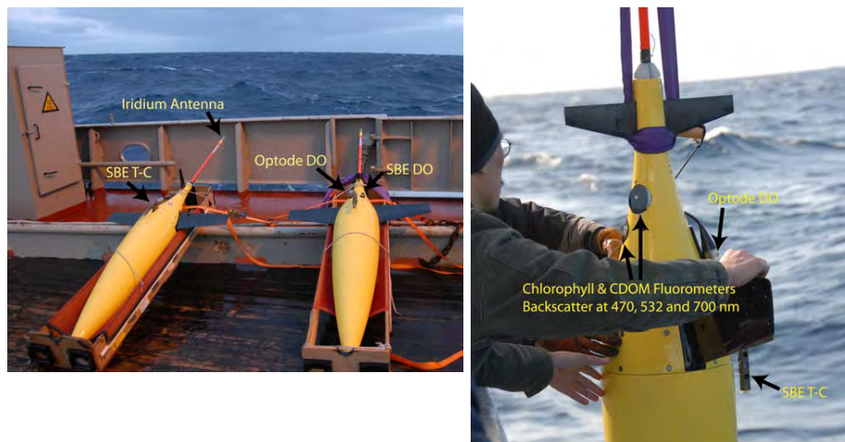
Figure S2: Seagliders used in NAB08 showing location of sensors.
