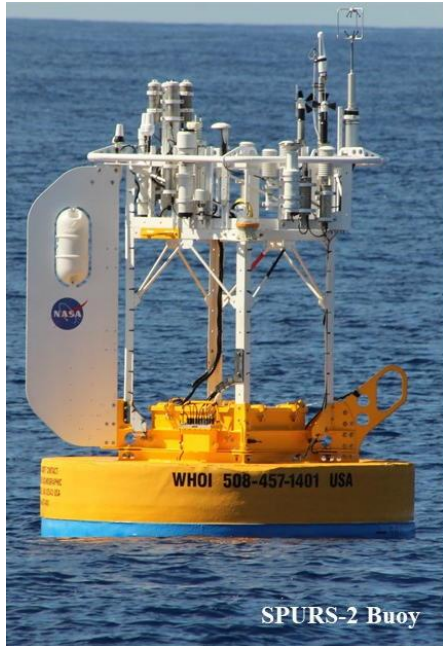
Figure 10: (left) The SPURS-2 central mooring with instrumentation at the upper right includes a sonic anemometer, infrared hygrometer, and sensors to remove buoy motion. The sensor package can directly measure the surface stress, sensible heat, and latent heat fluxes. (right) Time series of these fluxes showing bulk estimates in red and direct covariance (DC) fluxes in black. Good agreement is seen between the bulk and DC estimates, with the most significant discrepancies visible in the sensible heat flux. Photo by James B. Edson (WHOI).
