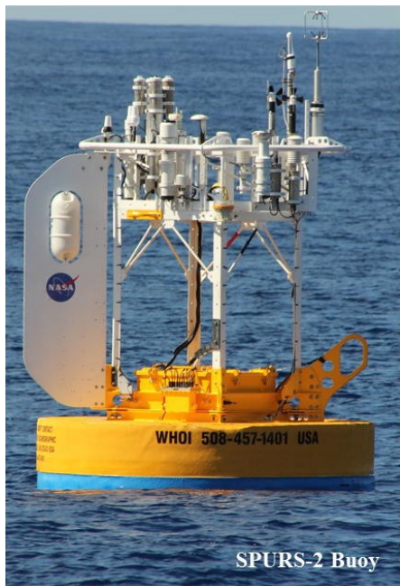
972 973 Figure 10: (left) The SPURS-2 central mooring with instrumentation at the upper right includes a sonic 974 anemometer, infrared hygrometer, and sensors to remove buoy motion. The sensor package can directly 975 measure the surface stress, sensible heat, and latent heat fluxes (See Clayson et al. 2019 for more details on 976 instrumentations). (right) Time series of these fluxes showing bulk estimates in red and direct covariance (DC) 977 fluxes in black. A good qualitative agreement is seen between the bulk and DC estimates, with the most 978 significant discrepancies visible in the sensible heat flux (Bigorre et al. 2013). The coincident measurements of 979 direct flux and bulk meteorology from SPURS-2 and prior field campaigns (e.g., CBLAST, DYNAMO, 980 CLIMODE, etc.) are being used for improving the bulk flux algorithm for turbulent heat flux transfer 981 coefficients. Photo by James B. Edson (WHOI).
