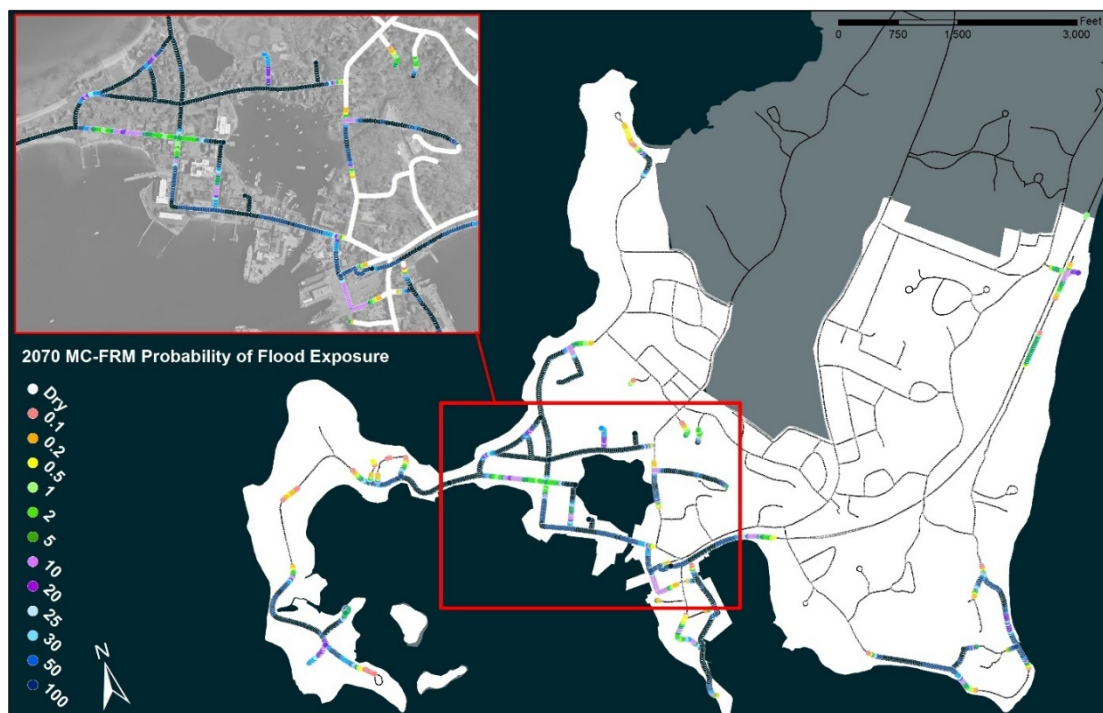
Figure 3-8 Roadway flooding projections – 2070
