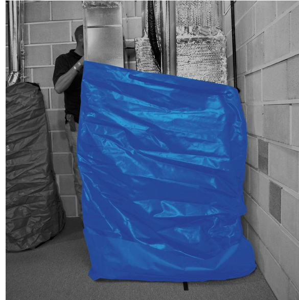
Utility flood covers are anchored to the floor and can be pulled up and secured around equipment in the event of a flood, assuming the equipment cannot be elevated and flooding is not excluded from the equipment room (floodproofing.com)
