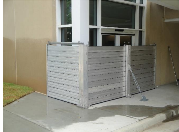
Flood planks are individual modular units that can be stacked between channeled columns on door and windows, and typically have a gasket to make the seal to wall and ground. The columns can also be strung across a span and linked together to form a fence ( psffloodbarriers.com )
