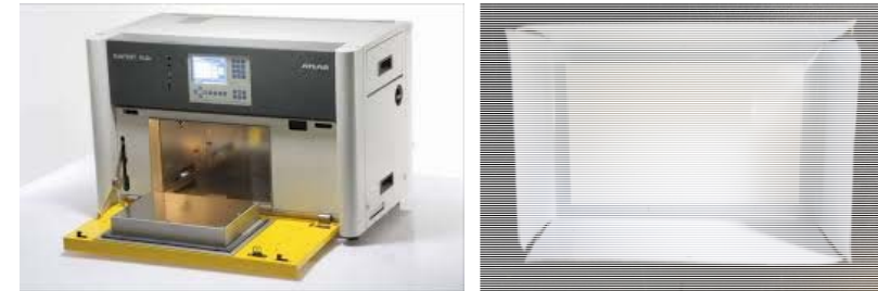
<Suntest XLS+(left) and rigid polystyrene sample placed on galvanized steel plate for UV exposure (right)>
