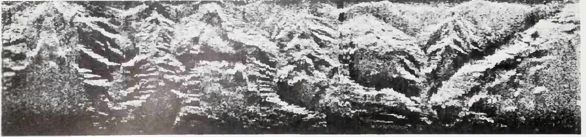
Figure 10. A side-scan sonar (4 kilohertz) inspection of the continental slope from the shelf edge south of the English Channel into the Bay of Biscay. Bright areas are shadows; dark areas have been ensonified. Note the marked diagonal channels and the intricate tributary system feeding the main diagonal canyons. The scene is approximately 12 kilometers from top to bottom and 48 kilometers long. (Courtesy Institute of Oceanographic Sciences, Britain)
