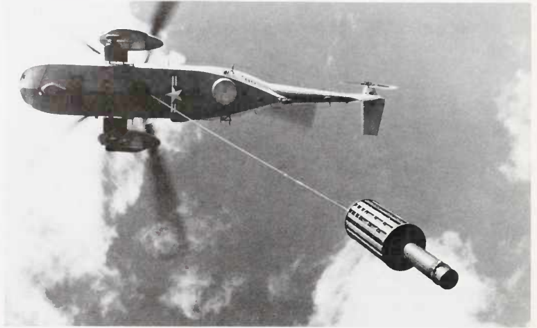
Figure 7. A Sea King helicopter lowering a sonar device during antisubmarine maneuvers in the Western Pacific. The helicopter is from the aircraft carrier USS Hornet. (Courtesy U.S. Navy)
