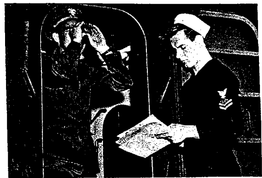
Figure 26. Procedure used in making bathythermograph observations. A. Inserting BT slide in slide holder. B. Swinging out gate boom. C. Level winding wire on drum. D. Taking bucket of water for surface temperature. E. Protecting winch with canvas cover. F. Labeling slides. G. Entering data on BT log sheets. H. Reading trace on BT slide.
