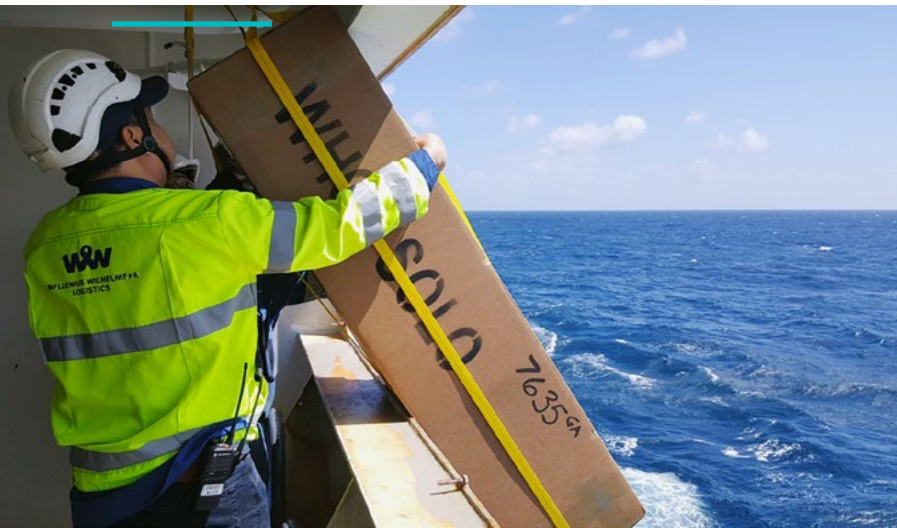
A crew member deploys an Argo float from the side of the ship. Once it enters the water, the biodegradable cardboard box quickly decomposes. (Photo courtesy of Capt. Erwin A. Augusto, master of M/V Tijuca )
