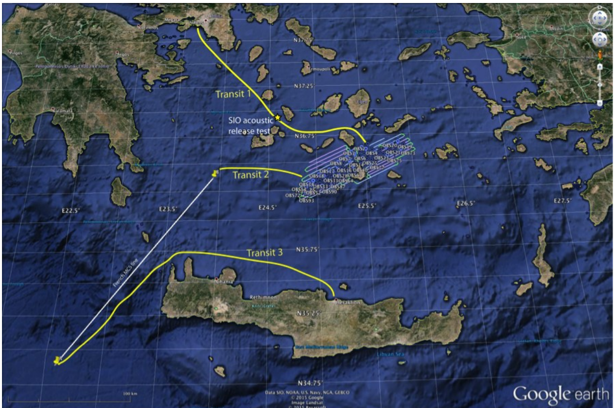
Draft plan for transits (yellow lines), offshore short period seismic deployment, and airgun shot profiles.
