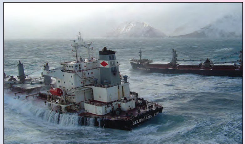
Figure B: Selendang Ayu on the north shore of Unalaska Island, Alaska, December 8, 2004. This image shows the two halves of the vessel after it foundered when the engines failed and towing attempts were unsuccessful. Six of the crew died in the accident and 336,000 gallons of fuel oil and diesel were spilled (NTSB 2006). This is the second largest spill in the region, following the Exxon Valdez spill in 1989. The spill and marine accident history of the Aleutian Island provides a guide for understanding the potential impacts of marine shipping incidents in the Arctic (CRRC 2009).
