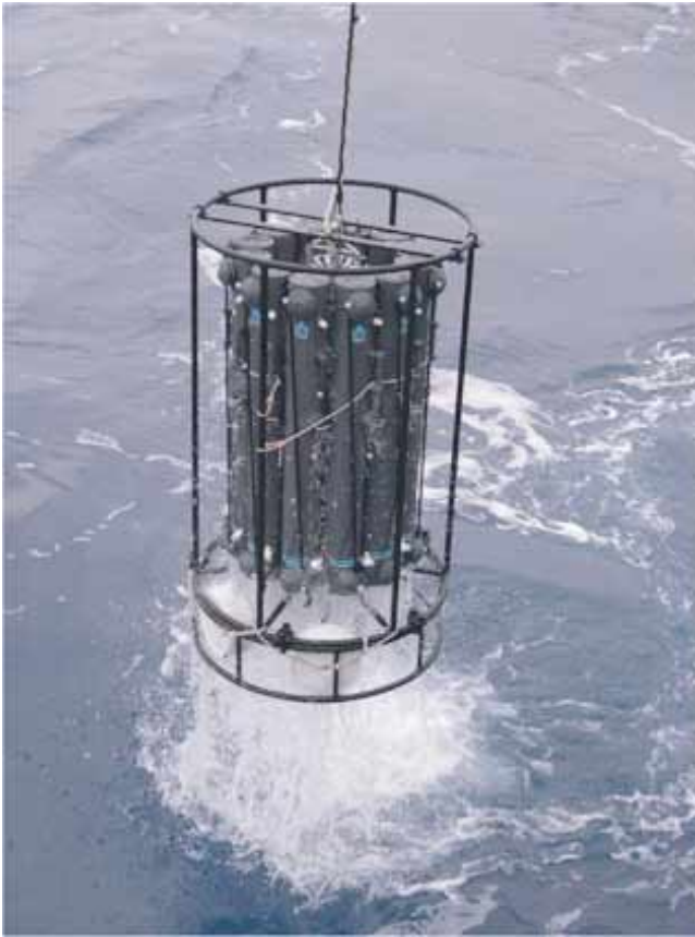
Figure 3. An example of one of several new TEI-clean sampling devices. This rosette consists of 12 Teflon™-coated Go-Flo bottles mounted on a powder-coated rosette frame with 0.38-inch 4-conductor, polyurethane-coated Kevlar line. To prevent contamination from the frame and auxiliary components, bottles are tripped from the deck while the package is moving upwards through clean water at low winch speeds (ca. 10 m/min). The system has been used to collect 12 samples in the upper 1100 m in less than 60 minutes. Sample bottles are removed from the frame and sub-sampled in a laboratory van with HEPA-filtered air. Figure provided by Chris Measures.
