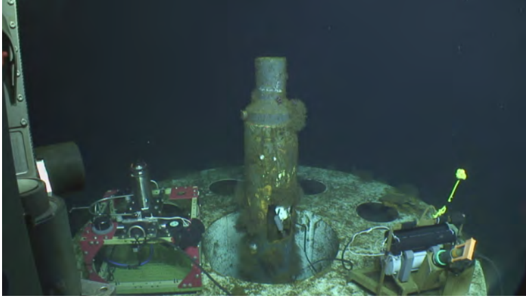
Photo 14. 8/25/2012 (RGB.20120825_055842_722) CORK 1025 showing final configuration of CORK logger (right) and optical modem (left).
