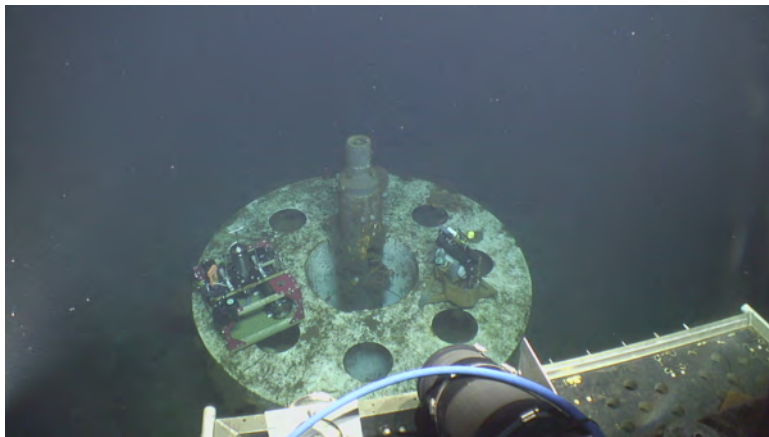
Photo 10. 8/25/2012 (RGB.20120825_042919_172) CORK 1025 with optical lander (left) and cork logger (right).
