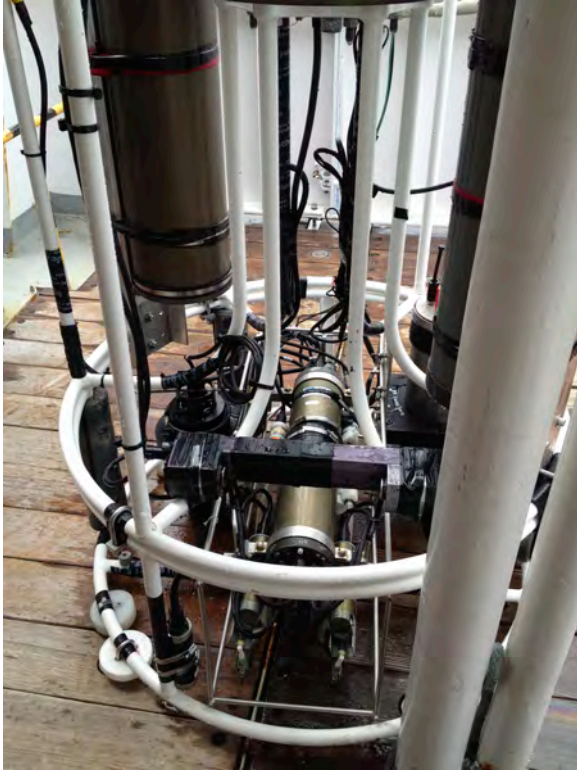
Photo 3. Photo showing seabird CTD, acoustic modem to left and transmissometer in foreground.
