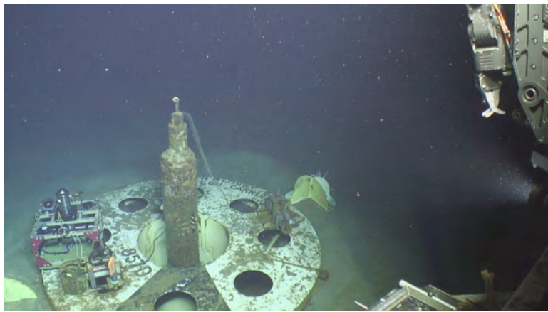
Photo 9. 8/24/2012 (RGB.20120824_123934_904) CORK 857D with optical lander and new cork logger (left) and old cork logger (right).
