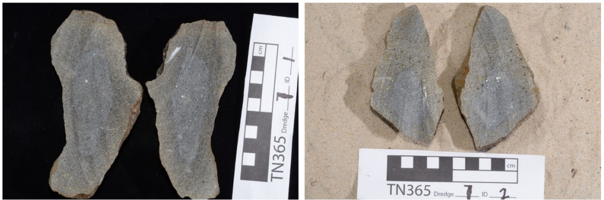
Fig. 13 D7-1: dolerite, vesicles filled with clay minerals indicative of very low-grade overprinting; yellowish colour in the outer parts due to greenschist-facies growth of epidote; D7-2; dolerite showing the same features as D7-1.
