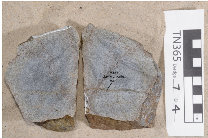
Fig. 15 Veins in dolerite. Irregular greenish and whitish clay + chlorite vein.
