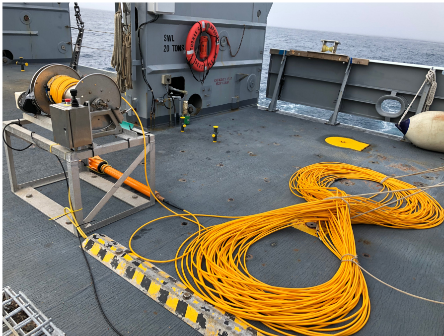
Figure 1. MISO SeaspY-2 surface towed magnetometer and winch.
