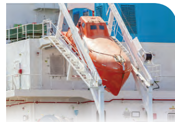
Exemplar enclosed freefall lifeboat in launch position on a slipway
