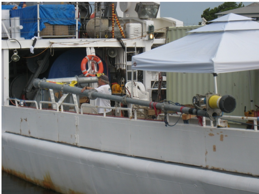
Figure A10 - USBL pole retracted and secured in the stowed position. To deploy, a crane is used to hold the near end, the assembly slides outboard relative to the base, and is rotated clockwise into the water where it is locked in the down position.
