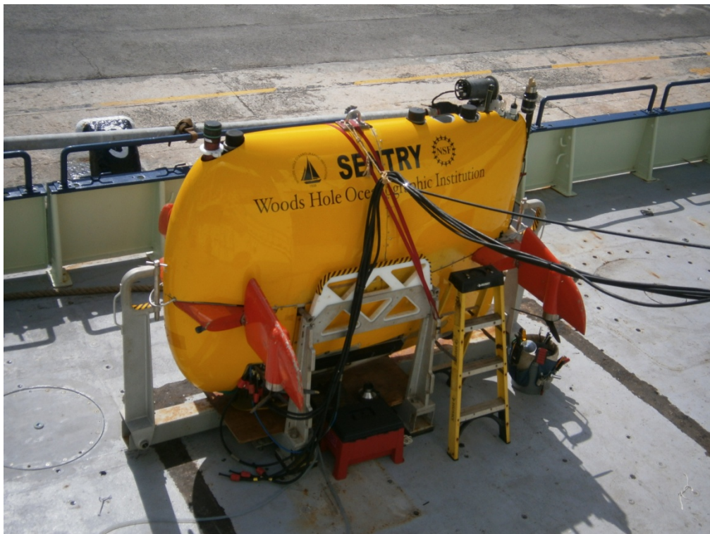
Figure A7. A picture of Sentry on the cradle on the deck of R/V Knorr. This picture has the Sentry umbilical and charge cables attached as well as the cooling lines. Note the cables running from the wall to the vehicle, the ample work room around the vehicle, and the proximity to the side of the ship relatively close to the water.
