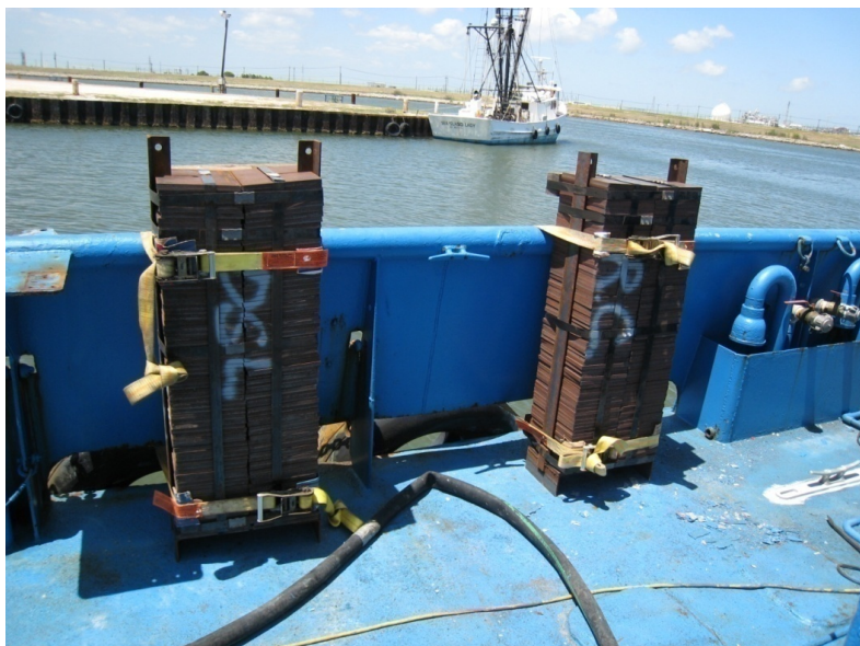
Figure A12 - Weight stacks secured to the side rail of a ship
