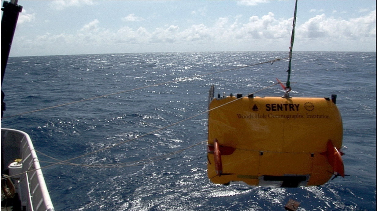
Figure A18 - Sentry continues to move outboard, the aft tagline is used to point the vehicle away from the vessel, then is slipped right before the vehicle enters the water. As soon as the pin is unloaded, it is pulled and the vehicle descends freely.
