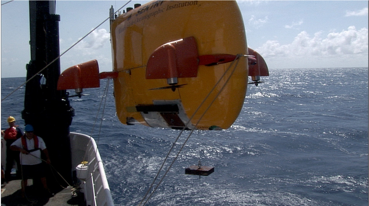
Figure A17 - As Sentry moves over the rail, the forward tagline is slacked and slipped.
