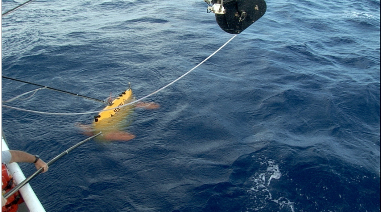
Figure A19 - As the vehicle drives towards the stationary vessel, the lift line for the crane is attached using a carbon fiber pole. The vehicle immediately drives full reverse and the pole is potentially used to fend the vehicle while the lift line is tensioned.
