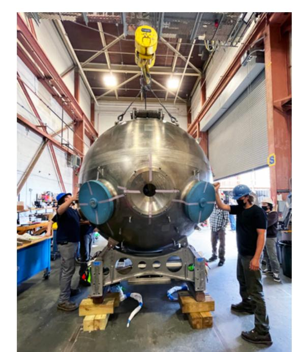
After stripping the sub down to its frame, the fabrication of new custom parts, and comprehensive maintenance on everything else, human-occupied vehicle Alvin is starting to take shape again. For a look at the upgrades that will come with the submersible's 6500meter depth rating, visit our overhaul page.
