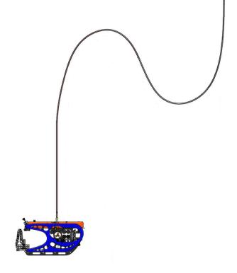
ENHANCED LOAD-CARRYING CAPABILITY MANAGES TORSIONAL FORCES TO PREVENT TWISTING & HOCKING ALLOWS FOR USE OF SMALLER WINCH
