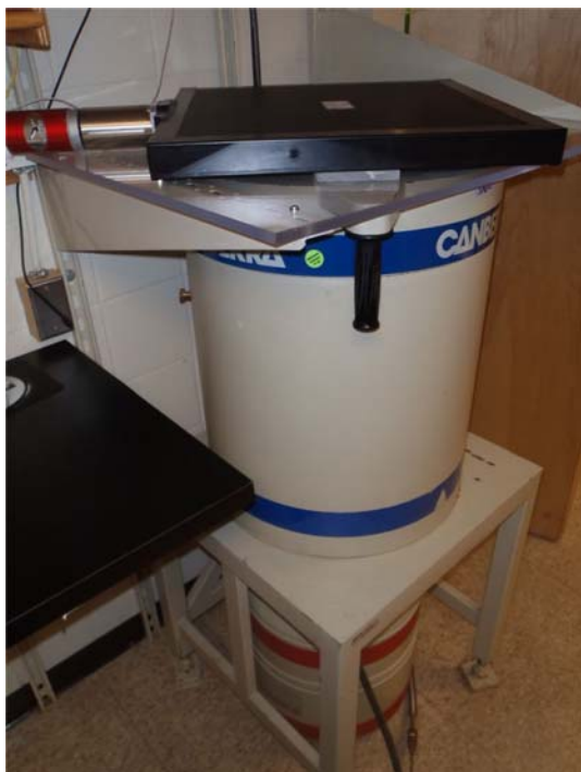
Fig. 3 Photograph of SAGe Well detector set up inside a 10 cm lead shield and a large area plastic detector used for cosmic-background suppression
