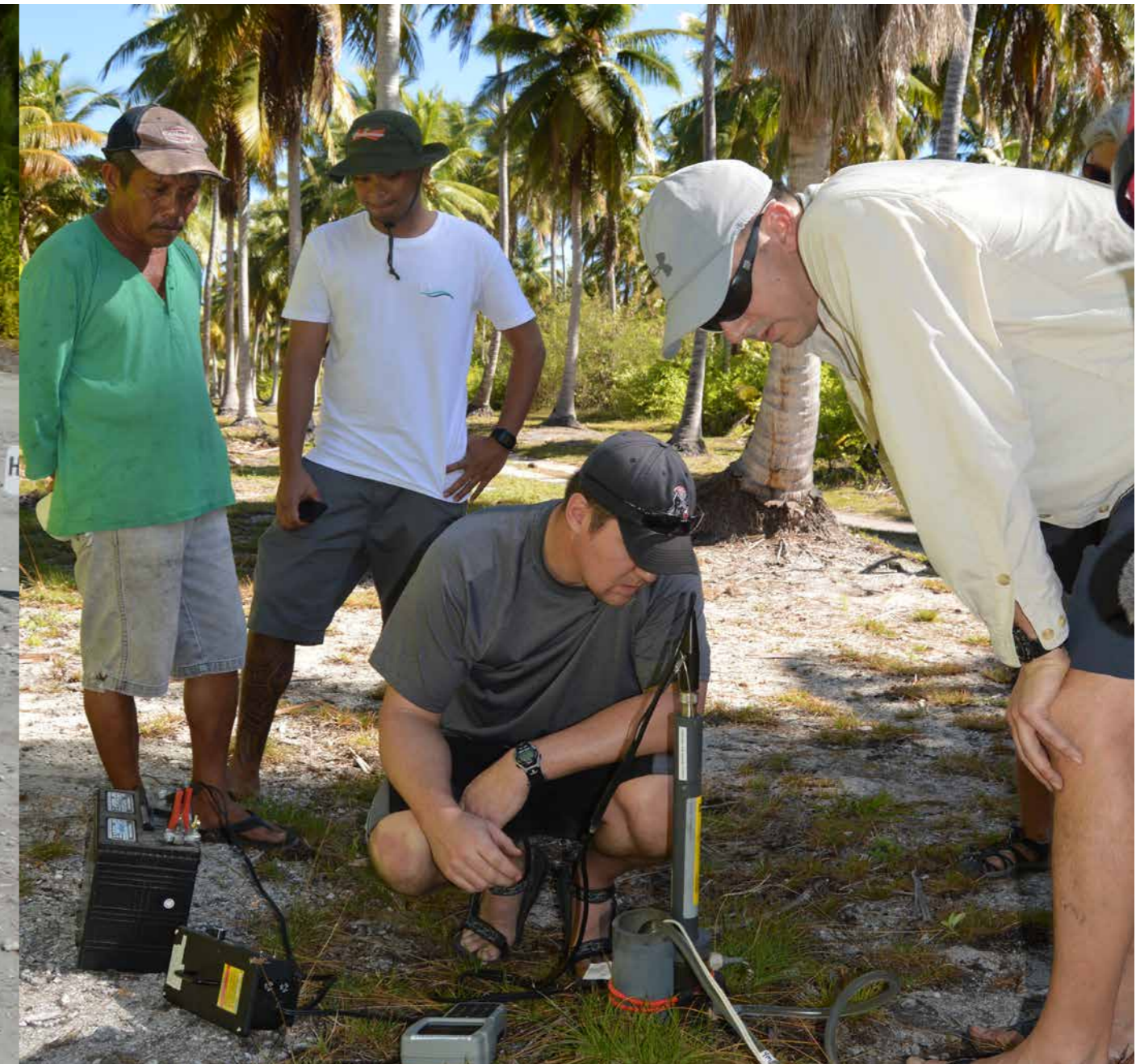
Matt Charrette and colleagues use a well pump to collect additional groundwater samples.
