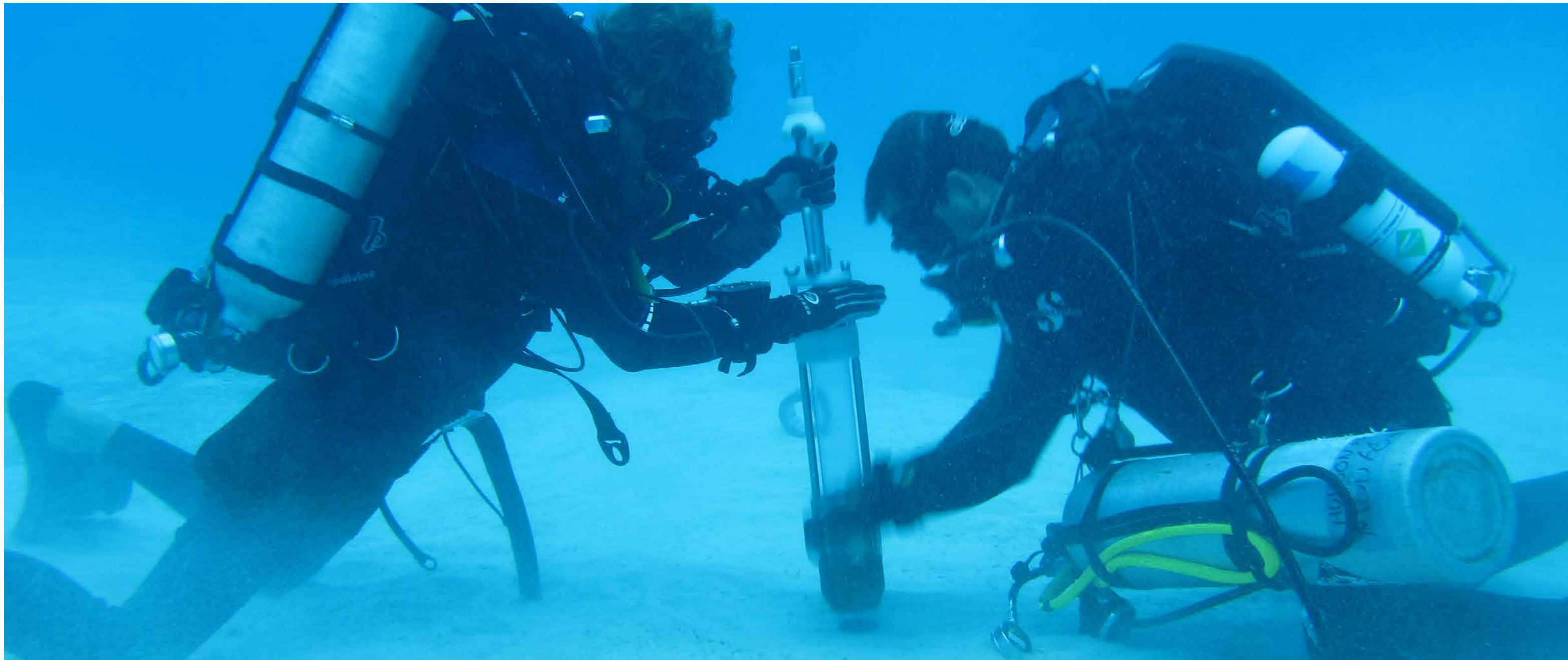
Hand driven "push cores" were taken by divers Steve Hudson and Walter Bubby at several sites in the Bikini and Enewetak lagoons to obtain a record of radioactive contaminants that remains associated with the seafloor sediments after the nuclear blasts.
