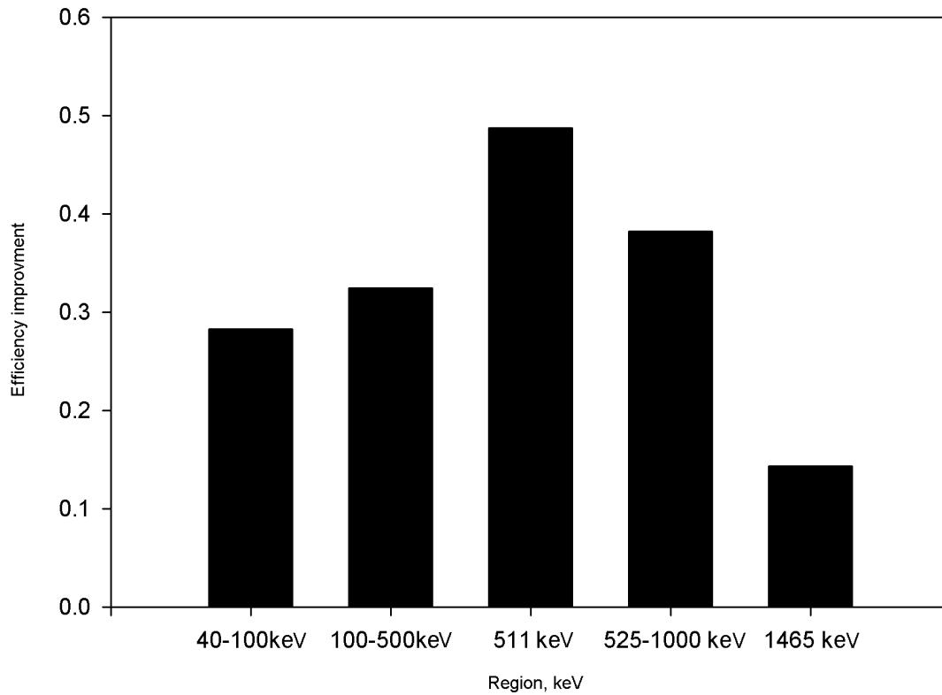
Fig. 6. Cosmic quard improvement, spectral comparisons broken into energy regions
