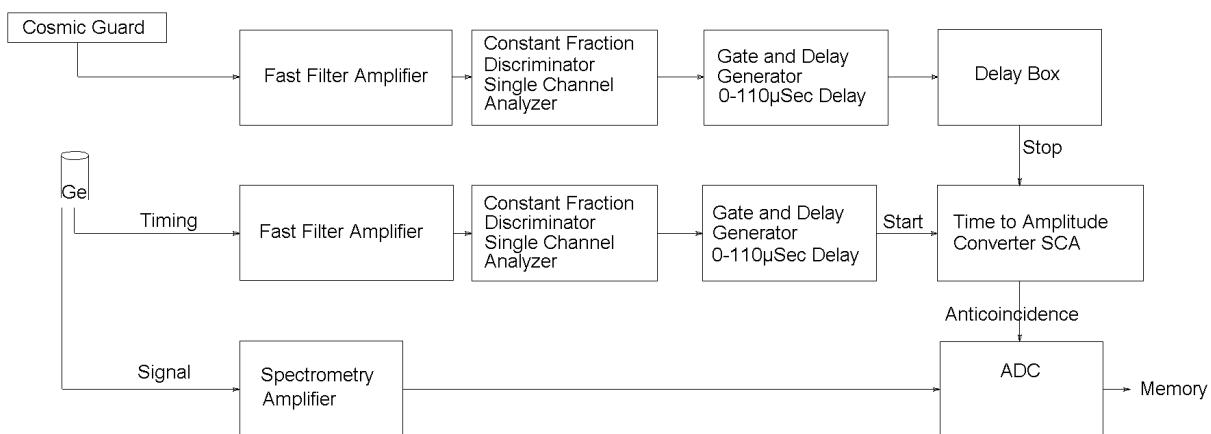
Fig. 2. Diagram of delay timing
