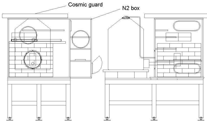
Fig. 1. Front view and side view of cosmic guard,  $\text{N}_2$  box and detector. The two upper circles on the front view are the glove ports. The nitrogen gas line connecting the Dewar and the detector chamber in the side view
