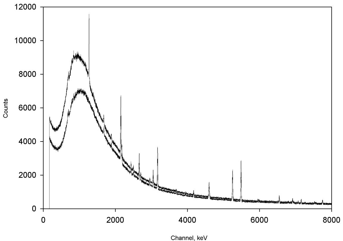
Fig. 4. Comparison one-hour spectra of unshielded HPGe on the 4th floor and ground floor of WHOI building
