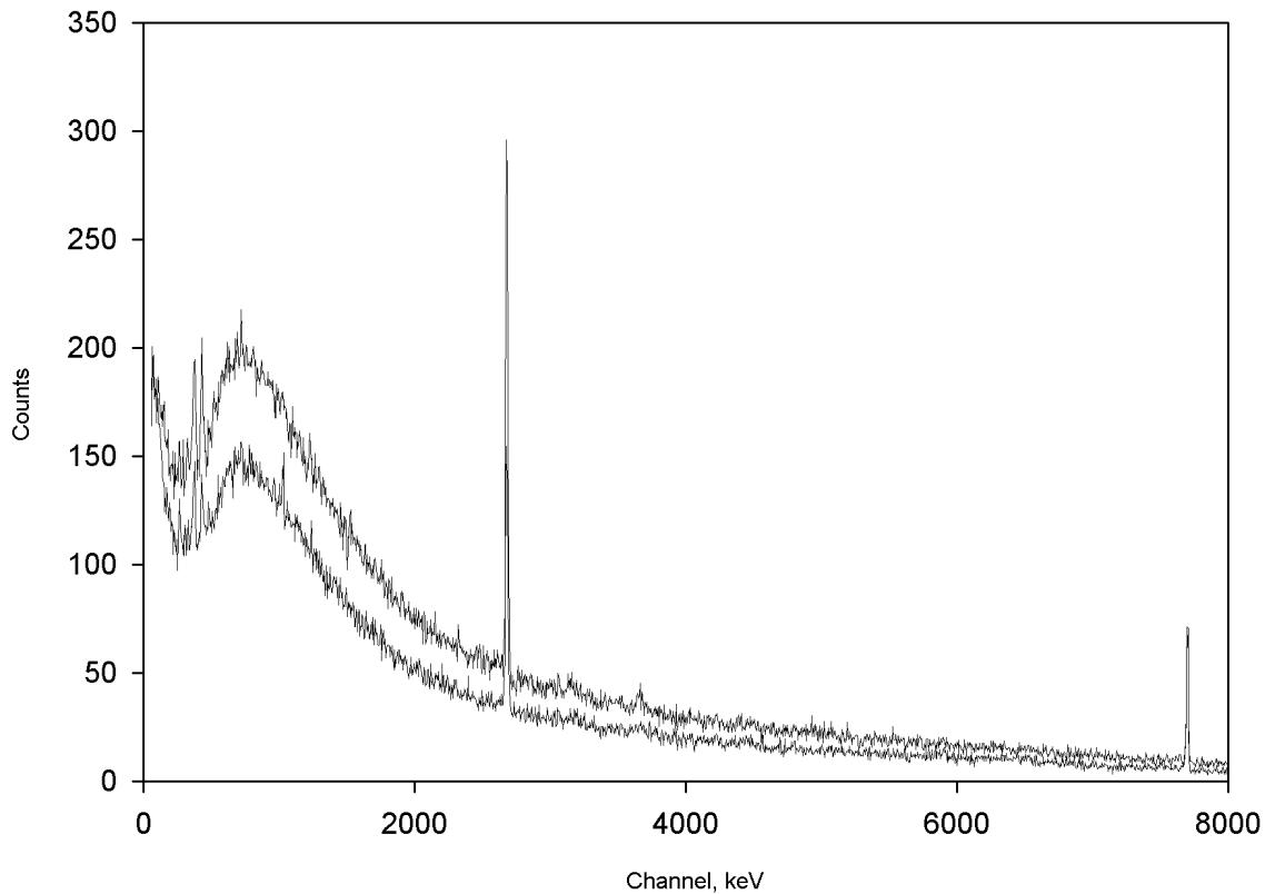
Fig. 5. Comparison spectra of four-day background count with cosmic guard disabled (upper) and enabled (lower)
