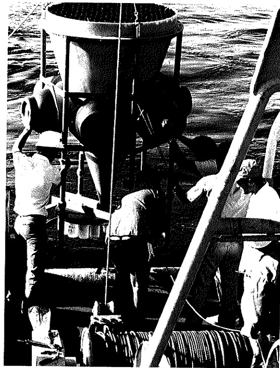
Figure 5. The Black Sea sediment trap on the stern of the research vessel.
