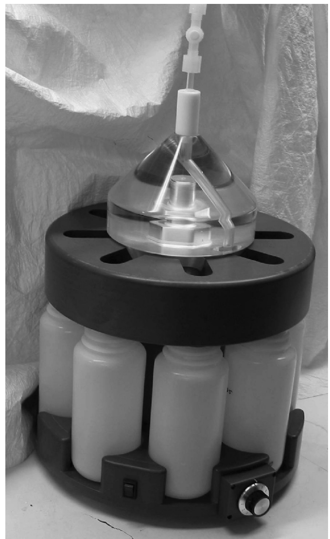
Fig. 2. Photograph of the custom wet splitting device used to generate equivalent subsamples of sediment trap material for a variety of analyses. Built for Café Thorium by Rich Zuck.
